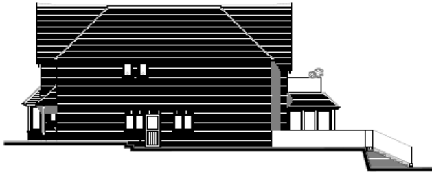
PROPOSED NORTH EAST (SIDE) ELEVATION PLOT 2 SCALE 1:100
